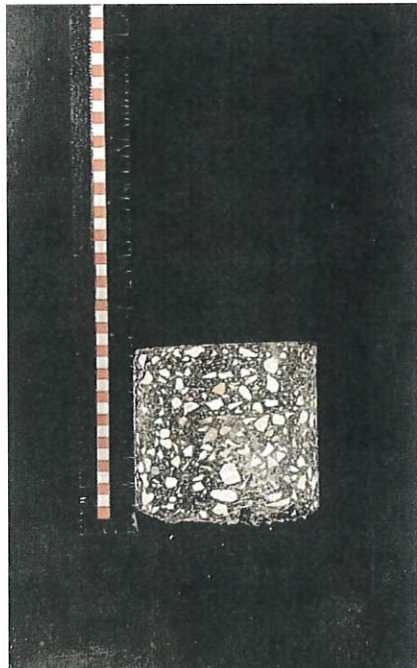
TH1 Full Depth of Pavement Ø = 150 mm
