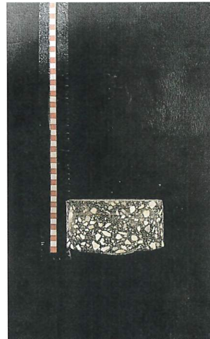
TH2 Full Depth of Pavement Ø = 150 mm
